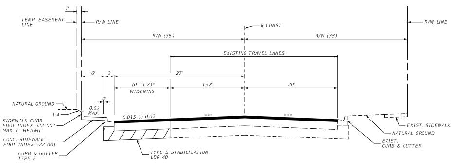
\* ACTUAL WIDTH OF BASE WIDENING MAY VARY DUE TO EXISTING PAVEMENT WIDTH. A UNIFORM WIDTH BASE WIDENING STRIP MAY BE CONSTRUCTED AT NO ADDITIONAL COMPENSATION.
