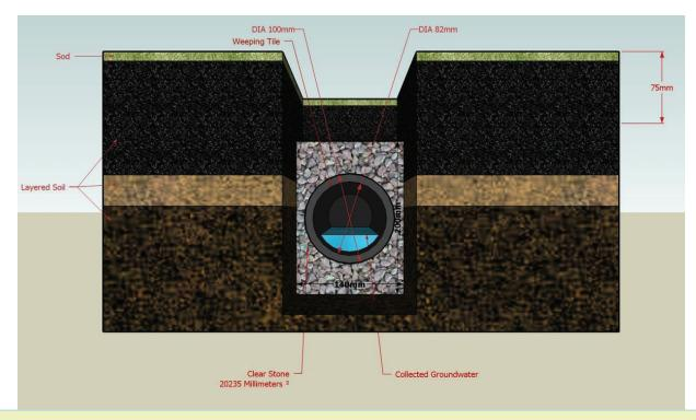
Figure 2-21: French drain. Source: Wikimedia Commons - www.commons.wikimedia.org/wiki/File:French\_drain\_diagram.jpg
