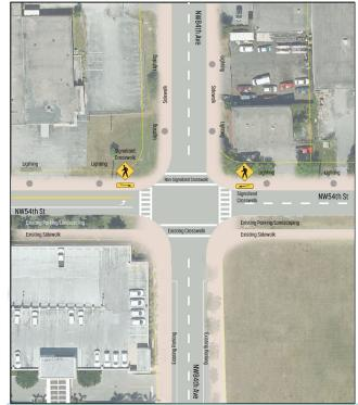
Figure 2-15: Potential Intersection and Right-of-Way Improvement Concept for NW 54th St and NW 84th Ave Note: Proposed improvements are meant as guidance; final roadway design may require modifications based on a more detailed engineering and design evaluation.
