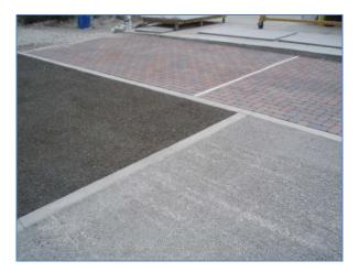
Figure 1 Pervious Pavement Sections at the UCF Research Facility
