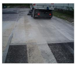
Figure 3 (a) Vacuum sweeping of sandy sediment loaded surfaces (b) vacuum sweeping of fine limestone dust loaded surfaces
