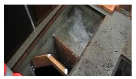
Figure 1. View of Inlet/Outlet Bay and a portion of the StormFilter Bay at 59 l/sec (2.1 cfs), 27 seconds into "instant-on" hydraulic test. Note that StormFilter Bay is still empty which indicates that the system is still in the process of filling.
