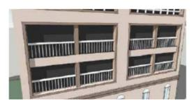
3. <u>Windowed opening</u>. The openings shall be framed, and mullions added to give the appearance of large windows.
