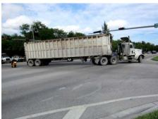
(Left): Turning radii are important at intersections; here, the diagram demonstrates spatial clearance in a turn. Issues arise with extended turn radii for trucks due to intersection design, as this may affect opposing vehicular and bicycling traffic making a
