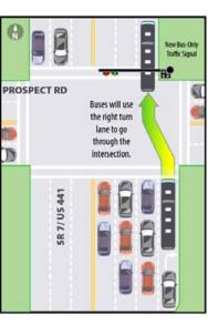
Different technology and traffic engineering techniques exists for bus priority signalization, which may be effect via detection devices as a bus approaches an intersection, allowing for a delayed red or an extended green (Left), by providing a separate green signal for the bus lane (Middle), or, as recently tested in Tamarac, FL in September 2014, by allowing buses to utilize a right turn lane to jump ahead in traffic (Right).
