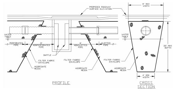
Figure 4-7 - Typical Exfiltration Trench
