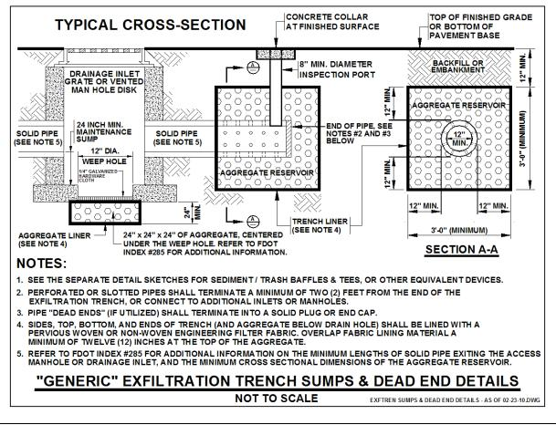
Figure 6-14 – Typical Exfiltration Trench Sumps and Dead End Details
