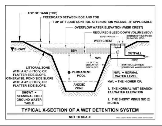
Figure 4-10 - Typical Cross-section of a Wet Detention System
