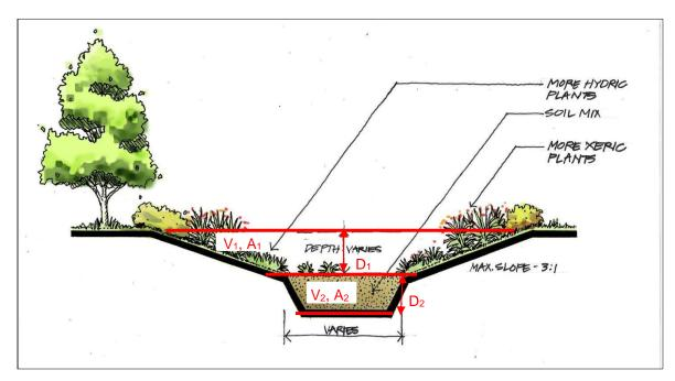
Figure 6-1 – Bioretention Basins Cross Section
