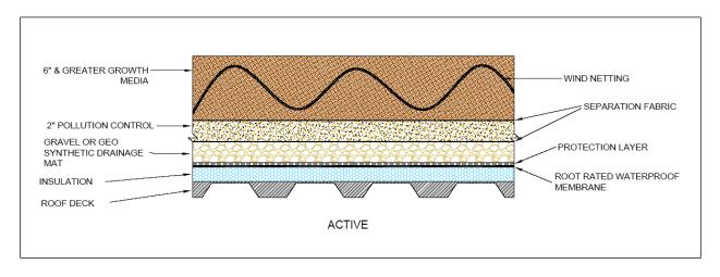
Figure 6-16 – Intensive Green Roof Section (Usually Active Function)
