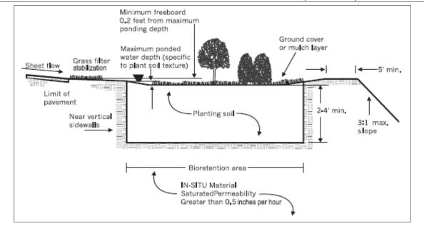
Figure 4-2 – Typical Bioretention Basin Cross-section
