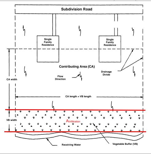
Figure 6-8 – Plan View Schematic of a Typical Vegetated Buffers
