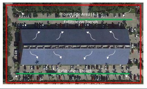
Figure 7-1 - Area Attributed to an Exfiltration Trench Length
