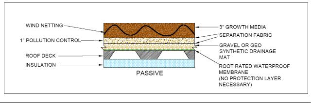
Figure 6-15 – Extensive Green Roof Section (Usually Passive Function)
