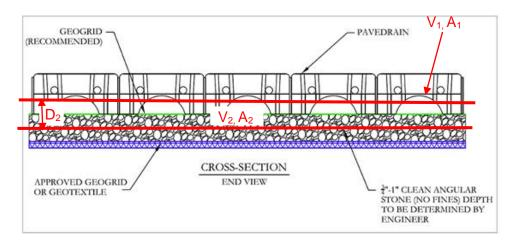
Figure 6-23 – Parking Stormwater Chambers Cross Section
