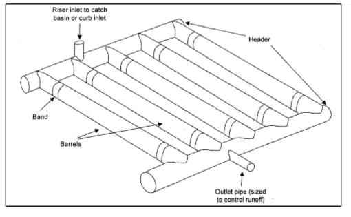
Figure 4-14- Example configuration of Parking Stormwater Chamber
