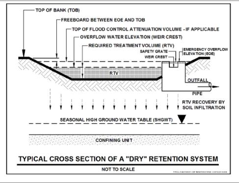
Figure 4-13 – Typical Cross-section of a Dry Retention System
