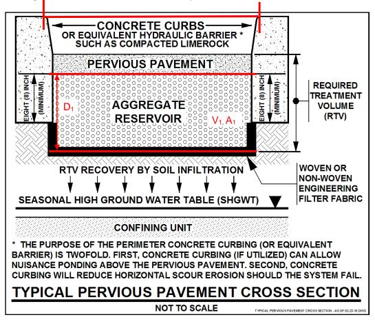
Figure 6-18 – Typical Pervious Pavement Cross-Section
