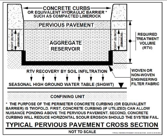
Figure 4-9 - Typical Pervious Pavement Cross-section
