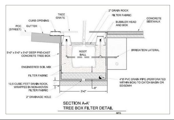
Figure 4-3 – Typical Tree Box Filter
