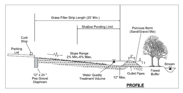
Figure 4-5 – Typical Profile of a Filter Strip
