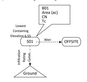
Figure 8-2 – Node-Link Schematic for a Model of a Development Site
