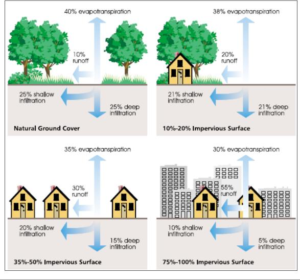
Figure 5-1 – Surface Runoff Variability with Increased Impervious Surfaces
