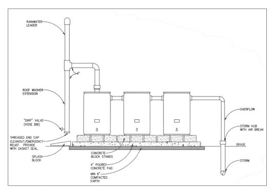
Figure 4-8 - Typical Profile of a Rain Barrel System
