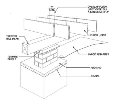
Figure 4-1 – Interior Detail of Example Pier
