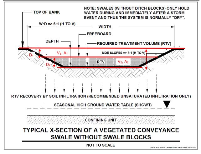
Figure 6-6 – Typical Cross-Section of a Vegetated Conveyance Swale
