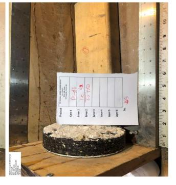
**Stabilized Subgrade? Light Brown Sand Stabilized Subgrade Thickness (in.) 12** Base Material Thickness (in.) 1 LR 5 Roadway BL NW 102ND AVE Station 43+38.34, 438.74 RT **Pavement Condition Good** Total Core Length (in.) 1 Cross Slope (%) 1 Cross Slope Direction In Crack \* Depth (in.) N/A Pavement Layer 3 S3 1 Longitude -80.358057 with Trace Limerock Latitude 25.832203 Core Date 7/1/2021 Rut Depth (in.) 0 Core ID PC-06
