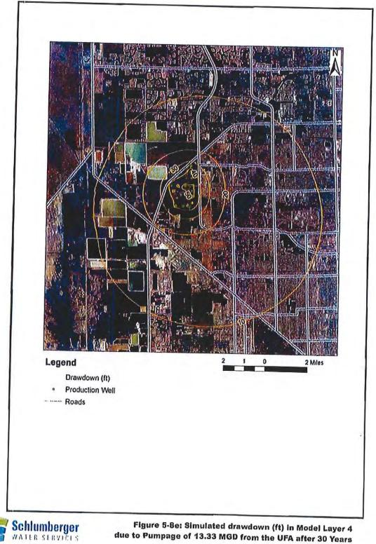
Figure 5-Be: Simulated drawdown (ft) in Model Layer 4 due to Pumpage of 13.33 MGD from the UFA after 30 Years
