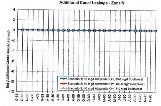
FIGURE 7 Total Net Additional Canal Scepage Relativo to Base Conditions
