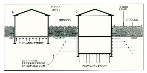
Figure 7-6. Hydrostatic pressures on a structure
