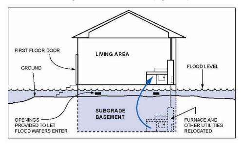
Figure 6-6. Wet floodproofing with a wet floodproofed subgrade basement
