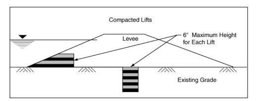
Figure 5-2. Levee construction
