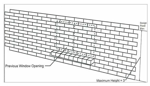
Figure 7-3. Permanently sealed opening
