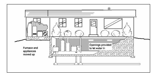
Figure 6-1. Wet floodproofed basement
