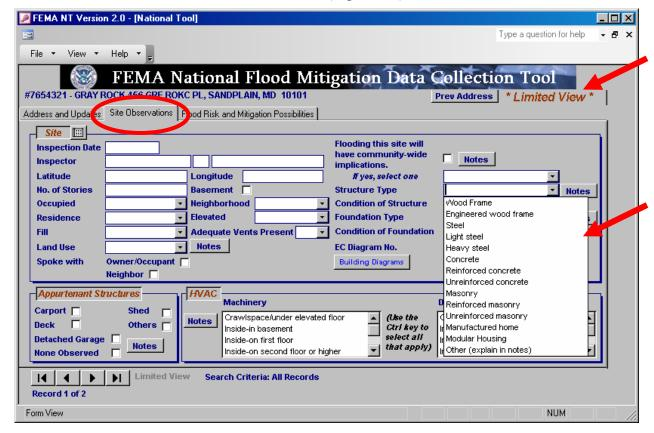
Figure 3-1. Site Observations tab - Structure Type menu
