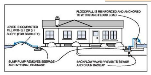
Figure 5-1. Structure protected by levee (on left) and floodwall (on right)
