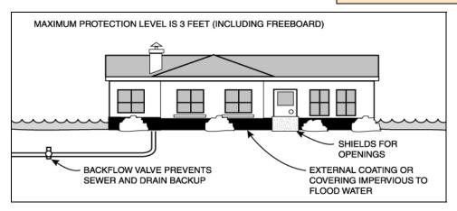
Figure 7-1. A typical dry floodproofed structure
