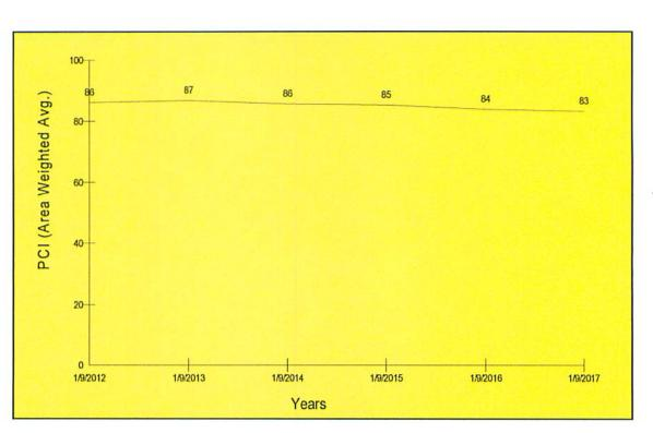
Figure 20-Average Weighted PCI After improvement Based on Critical PCI Method
