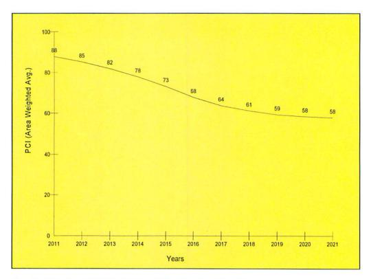
Figure 14-Predicted PCI for Tertiary "T" Pavement Sections
