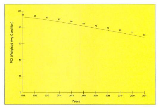
Figure 12-Predicted PCI for Primary "P" Pavement Sections
