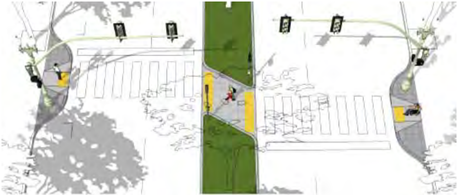
Midblock crossings allow for safe and convenient passage for pedestrians, and can be developed to enhance the visual environment.
