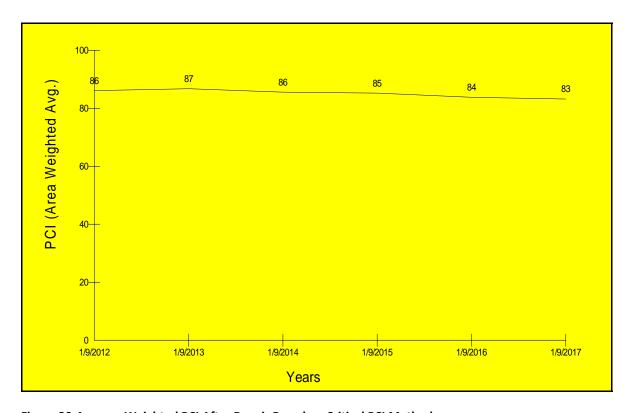
Figure 20-Average Weighted PCI After Repair Based on Critical PCI Method
