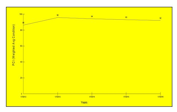
Figure 16-Average Weighted PCI After Repair Based on Minimum PCI of 86
