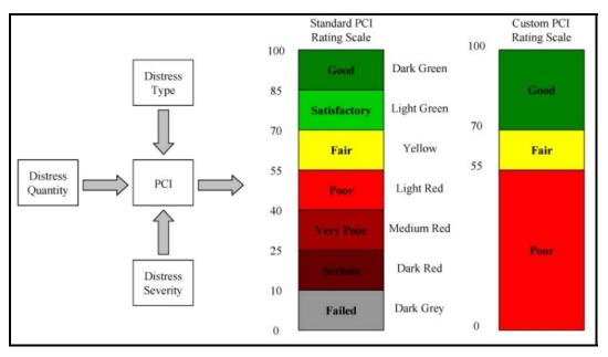
Figure 2-Pavement Condition Index Rating Scale
