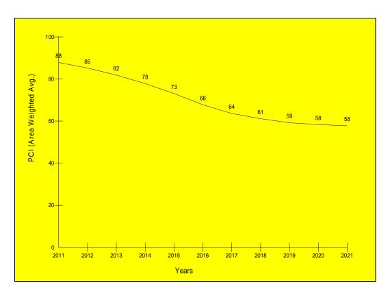
Figure 14-Predicted PCI for Tertiary "S" Pavement Sections
