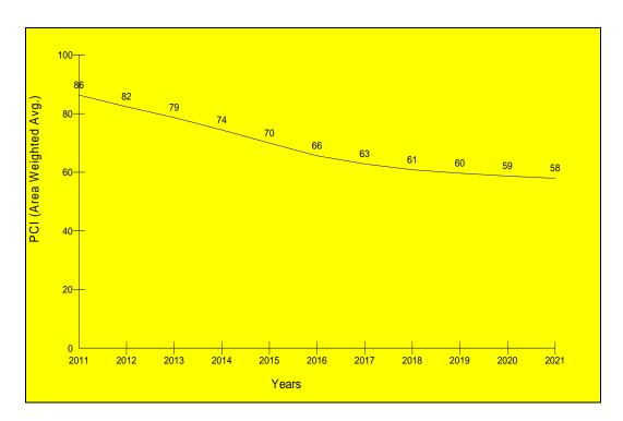
Figure 13-Predicted PCI for Secondary "S" Pavement Sections
