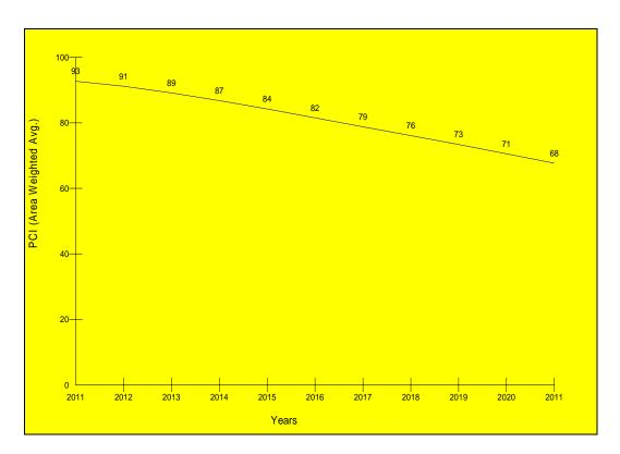
Figure 12-Predicted PCI for Primary "P" Pavement Sections
