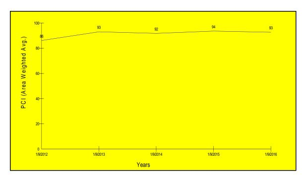
Figure 18- Revised Average Weighted PCI After Repair Based on Minimum PCI of 86
