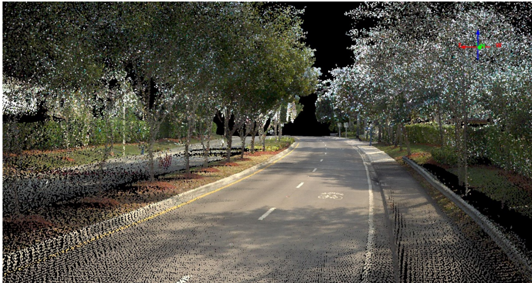
Digital Twin - Point cloud analysis 3d model , measurements accuracy 2 cms
