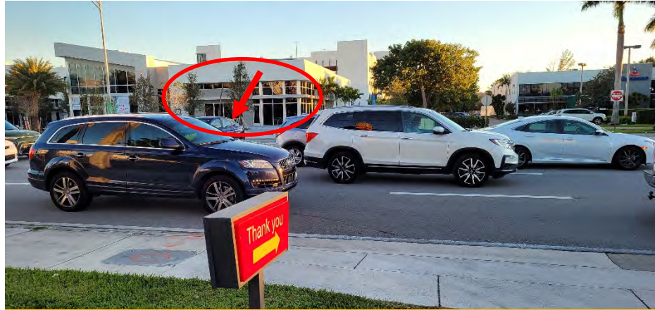
Photo 46: Eastbound vehicle making a U-turn among stopped westbound vehicles at Median Opening #4
