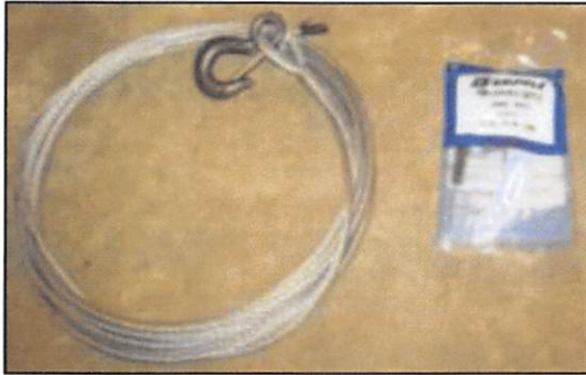
40' winch cable rated to 7,000lbs
